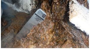
**The Omni Stainless Steel Combs** include markings for depths ranging from .002 to .125 inches with notations of *Acceptable, Cleaning Required* and *Critical Depth* as listed in the NFPA 96 2014 edition FIGURE A.11.6.2
